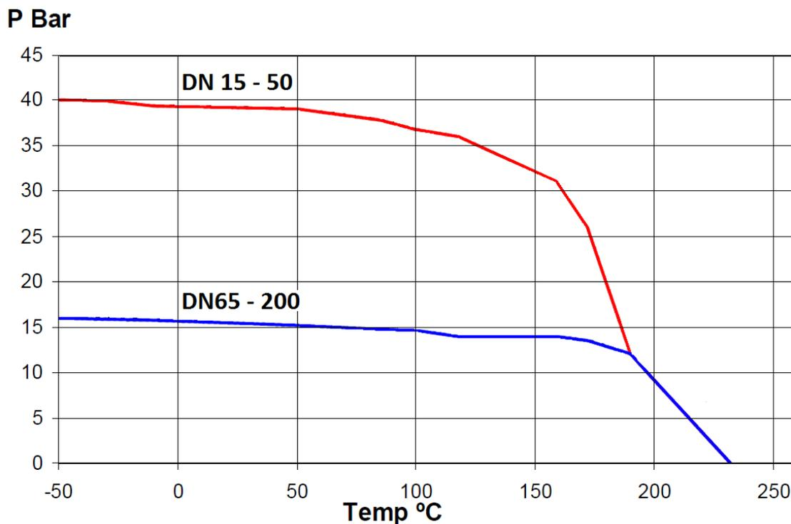
**ROBINET A TOURNANT SPHERIQUE 2 PIECES A BRIDES PN 16/40 ICP DIN 3202 F4/F5**
